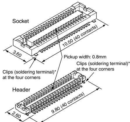
\* Clips for preventing the solder joints from being removed
